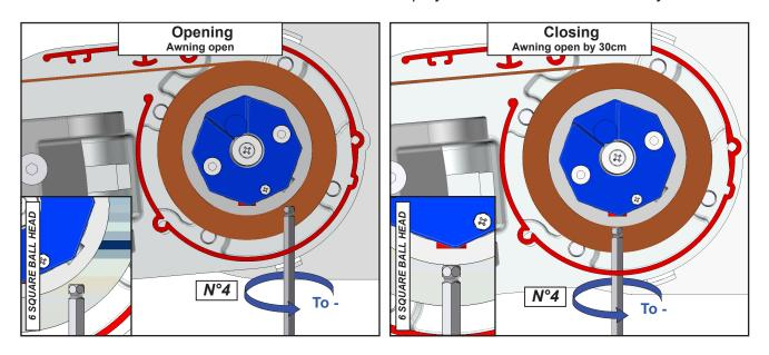
Limit switch: Turn the screw towards the '+' for more closing or opening, towards the '-' for less closing or opening. Carry out a test to validate the stop. Warning: the motor will go into thermal protection after 2 successive lifts and 1 successive lowering.
