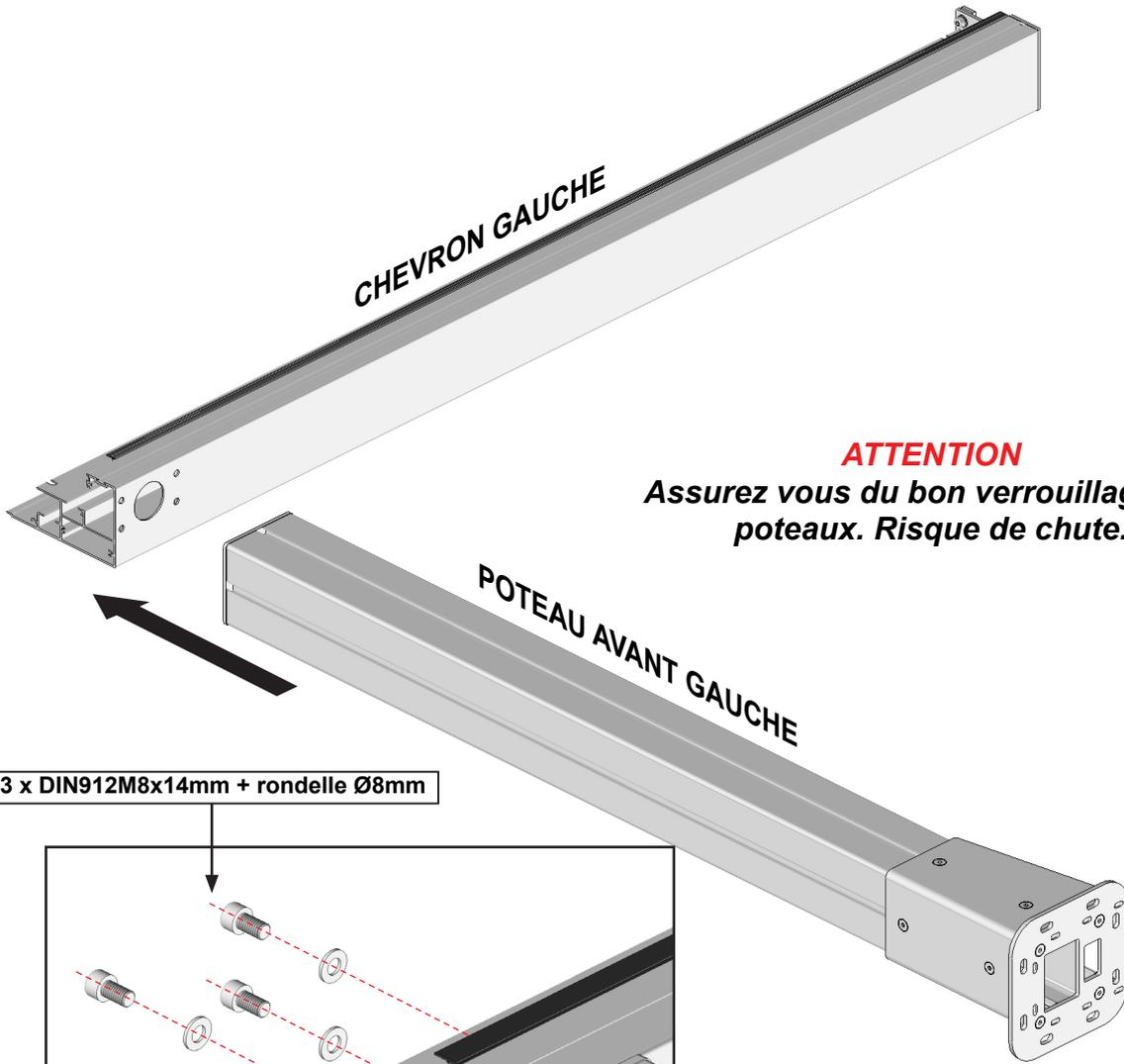
3 x DIN912M8x14mm + rondelle Ø8mm
