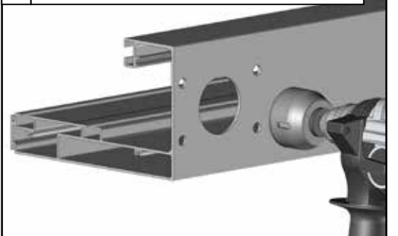
C Drill 1xØ50mm + 4xØ9mm.
